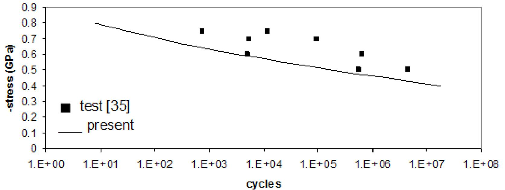
Tension-Torsion case (tension=torsion and  $R=0$ ) for woven glass fabric
