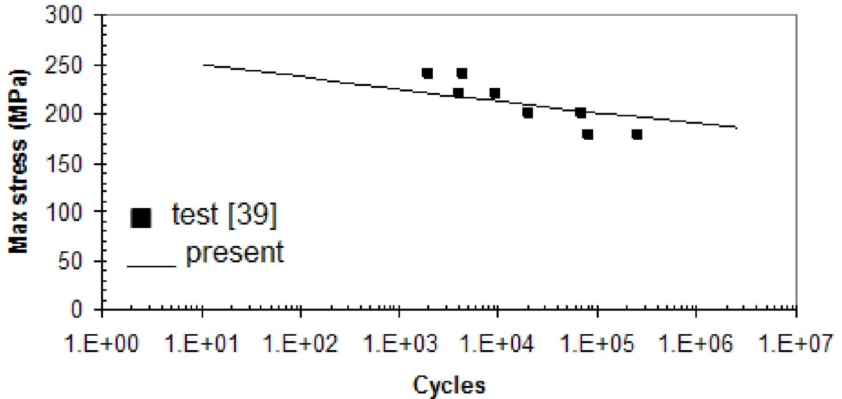
Tension-compression fatigue (R=-1) of [02/±45/02/±45/90]<sub>s</sub> BMI laminate
