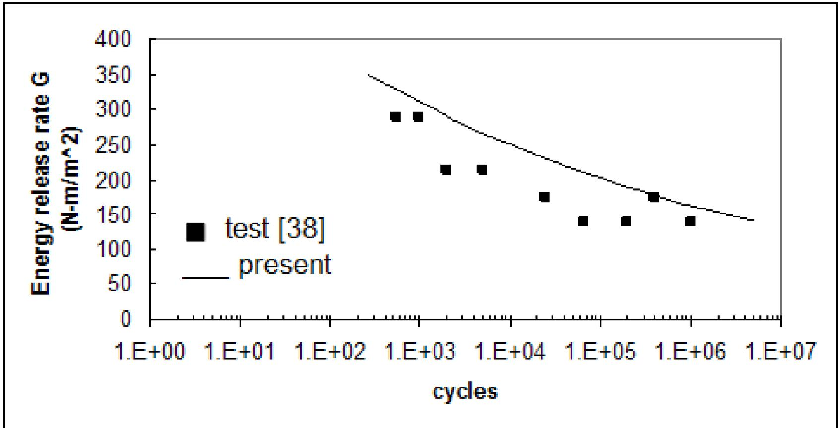
Onset of delamination for quasi-isotropic glass/epoxy (R=0.1)
