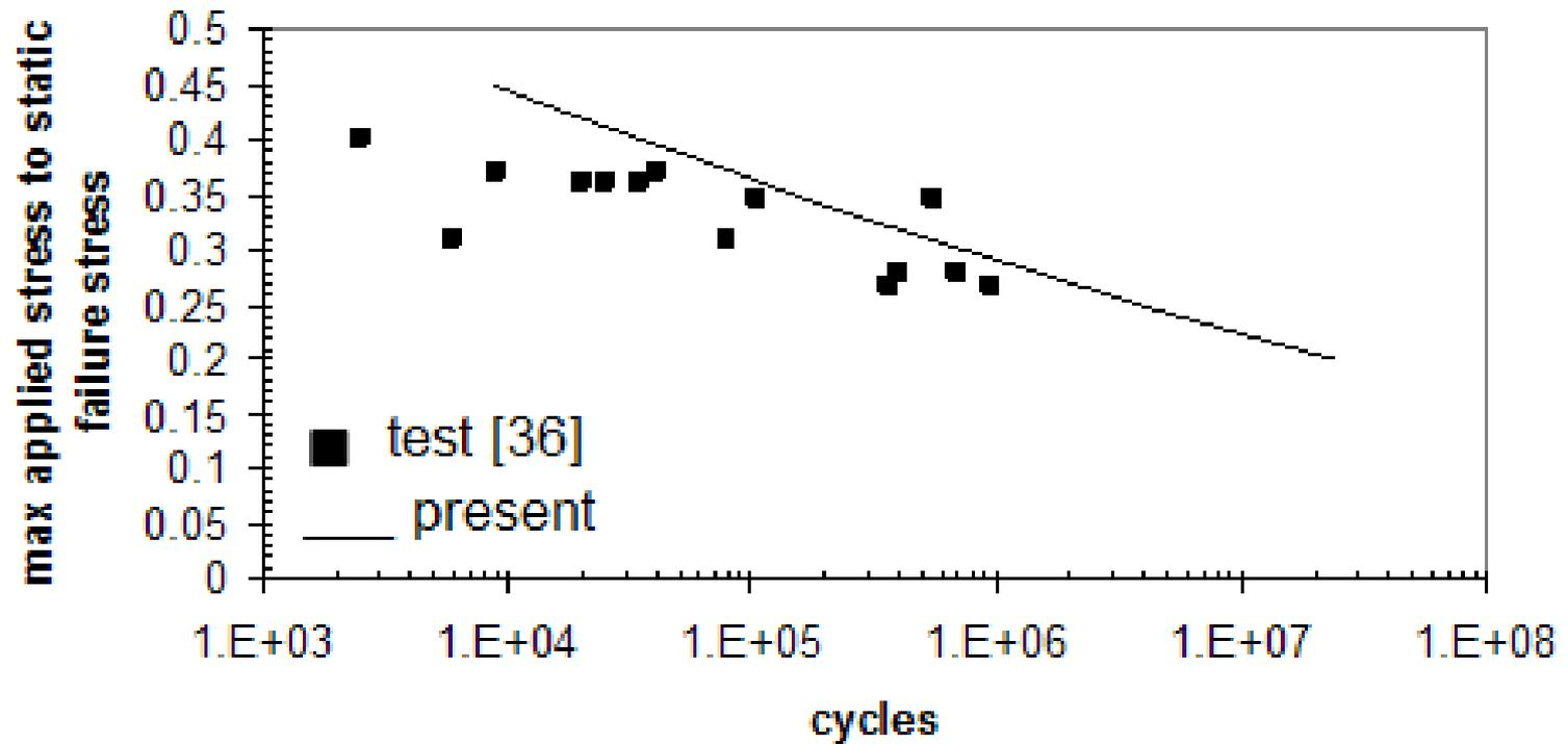
Onset of delamination load for skin/stiffener configuration (R=0.1, IM6/3501-6 material)
