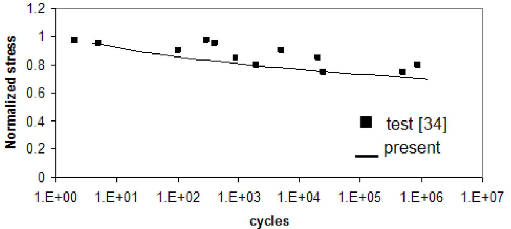
Tension-tension fatigue for  $[(\pm 45/0_2)_2]_s$  T800/5245
