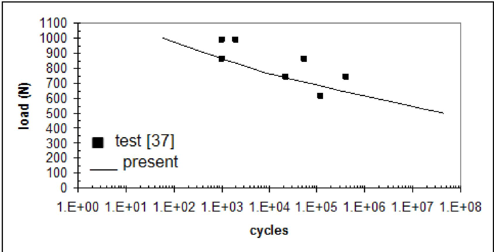
. Onset of edge delamination for [35<sub>2</sub>/-35<sub>2</sub>/0<sub>2</sub>/90<sub>2</sub>]<sub>s</sub> AS4/PEEK (R=0.1)
